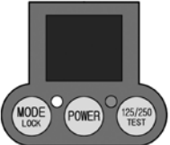
Error : Blank LCD screen Possible Cause : CPU electrical malfunction or battery problem Solution : Replace battery pack or press reset button to restart the lubricator. If the problem persists, contact your supplier.
