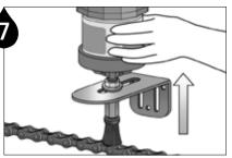
When the selected dispensing period of the Pulsarlube EO has completed, remove the lubricator from the application.
