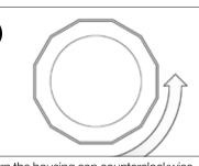
Turn the housing cap counterclockwise to unscrew the cap.
