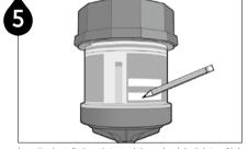
Log the installation date and the scheduled date of lube cycle completion on the label of the Pulsarlube EO. Note Please note there is a delay before the unit starts dispensing oil. It can take up to 3 weeks for enough gas to generate to start dispensing depending on the monthly setting and installation conditions.
