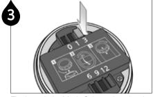
Firmly push the Mode Selector into the slot of the desired dispensing period.
