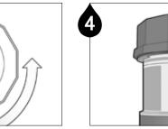
Put the cap back on and turn it clockwise until the cap is securely locked in place.
