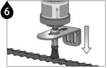
Install the unit on the lube point using appropriate adapters.
