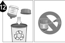
Dispose of remaining plastic components complying with local regulations for recycling. Warning Do not cut, puncture, or reuse lubricator. Avoid high backpressure. The backpressure at the tip of lubricator must be under 5bar.
