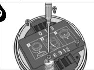
Unscrew to remove the battery cover.
