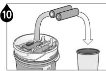
Remove the batteries.
