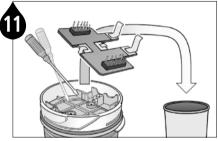
Using a hand tool such as a flat-head screwdriver, detach the PCB from the unit.
