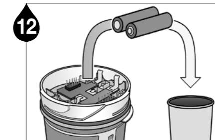
12 Remove the batteries.
