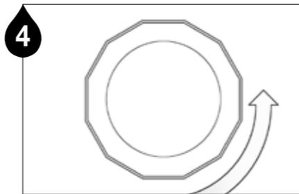
4 Turn the housing cap counterclockwise and unscrew the cap.
