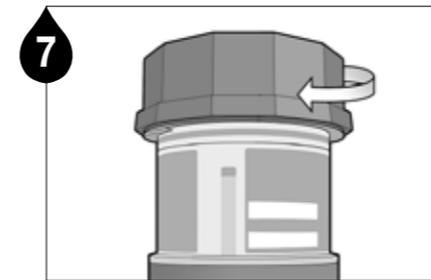
7 Screw the housing cap on the body.
