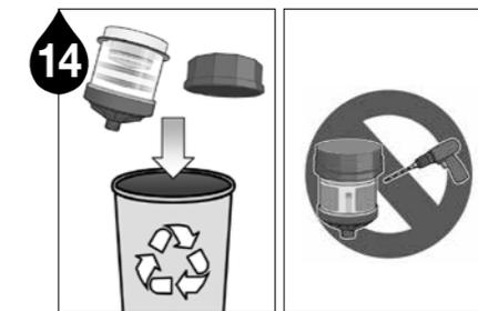
14 Dispose of remaining plastic components complying with local regulations for recycling. **Warning** Do not cut, puncture, or reuse lubricator.
