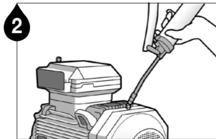
2 Ensure a clear passage using a manual grease gun. **Note 1** Remove any hardened grease by purging the lube point with a manual grease gun. **Note 2** The grease in the equipment and the grease contained in the unit must be the same or compatible.
