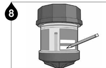
8 Note the installation date and the scheduled date of lube cycle completion on the label of the Pulsarlube E. **Note** Please note there is a delay before the actual dispensing starts. It may take up to 1-3 weeks for enough gas to be formed depending on the dispensing setting & installation condition.
