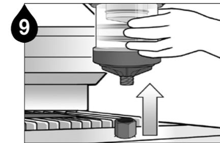
9 When the selected dispensing period of the Pulsarlube E has completed, remove the lubricator from the application.
