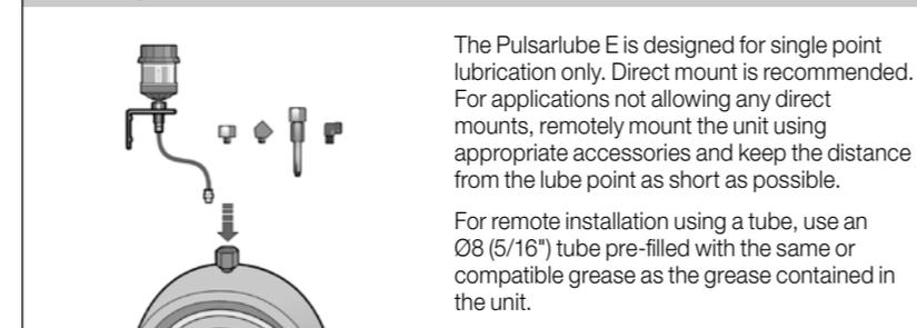
The Pulsarlube E is designed for single point lubrication only. Direct mount is recommended. For applications not allowing any direct mounts, remotely mount the unit using appropriate accessories and keep the distance from the lube point as short as possible.
