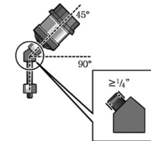
For remote installation using an Ø8 tube, keep the maximum distance at 1m (3ft) or less.
