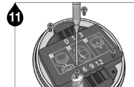
11 Unscrew the screws to remove the battery cover.
