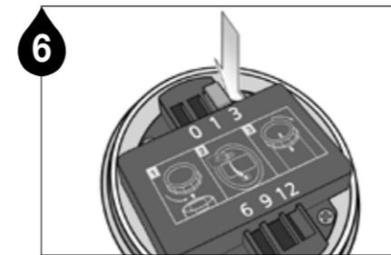
6 Firmly push the Mode Selector into the slot of the desired period.
