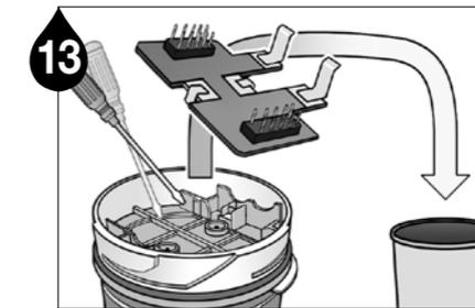
13 Using a hand tool such as a flat-head screwdriver, detach the PCB from the unit.
