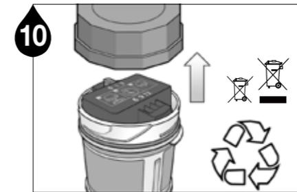
10 The Pulsarlube E is an eco-friendly product that can be disposed of separately. Turn the housing cap counterclockwise to disassemble the product for proper disposal.
